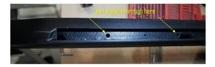
4. After all M-Power Lights are installed in the mount feed the pigtails through the 3/8" holes you drilled in the running board being careful not to pinch any wires and lay the mRUNNER in the hole.
