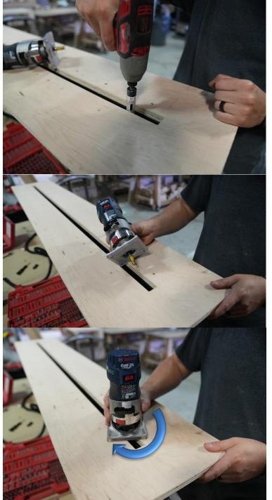
**5.** Drill a 5/8" hole into the end of the edge of the running board inside the jig hole.
