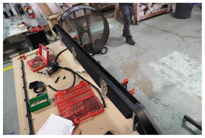
**8.** Inspect the hole and make sure it is fully cut out flush with the jig then remove the jig and vacuum out the plastic shavings leaving the Running board clamped to the table.
