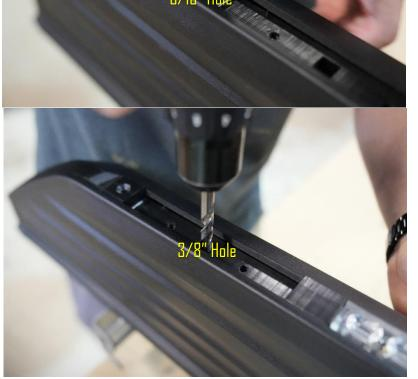
**2.** Drill through the center pigtail holes with a 3/8" drill bit through the back of the running board.
